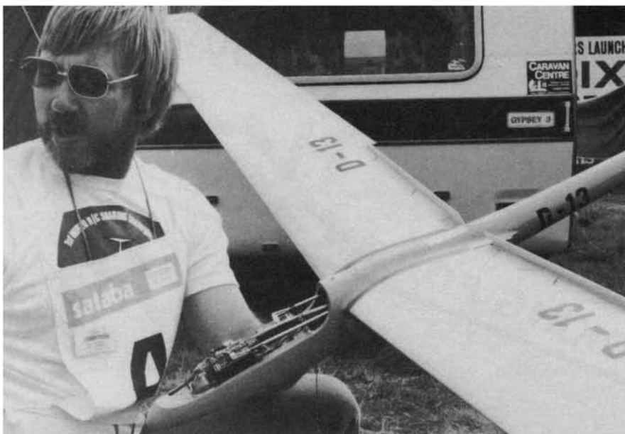
Ralf Decker, European F3B Champion, with his much photographed original. The deployed flaps/brakes reveal carbon filament lines that reinforce foam core. Balsa sheet fiberglassed.
