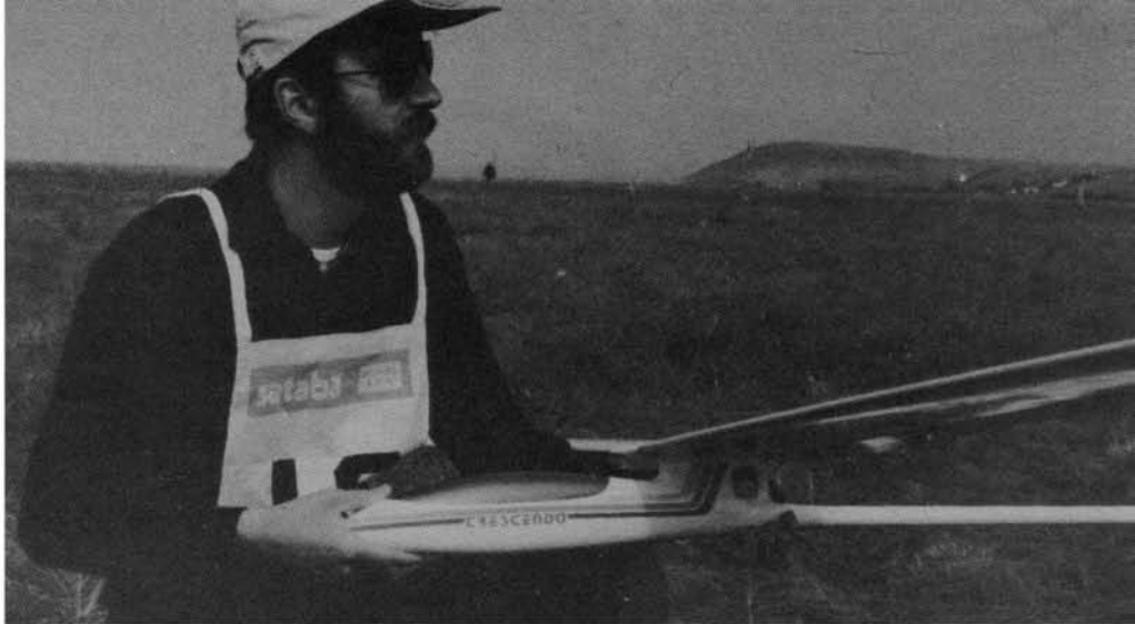
World renowned Eugenio Pagliano of Italy and his latest design. Wing is pylon mounted, flap servo in pylon. Wind tunnel tested, Crescendo's design has been proved aerodynamically sound.
